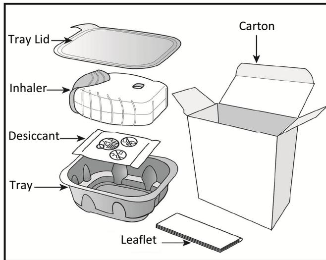
The plastic ELLIPTA inhaler is packaged in a tray, with a peelable foil lid. **Do not remove the foil lid until you are ready to use the inhaler.** Peel back the lid to open the tray.
