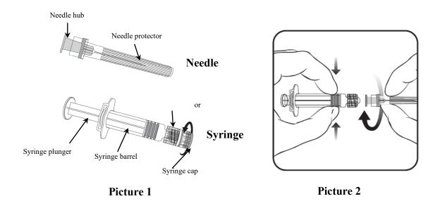
Always hold the syringe by the barrel, not by the syringe plunger or the Lucr Lock Adaptor (LLA), and maintain the needle in the axis of the syringe (as illustrated in picture 2). Failure to do this may cause the LLA to become distorted and leak.
